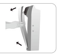
1 With the thumb against the front panel, right hand into the gap at the front panel of the machine connected to the hands and gently clawed front panel to open the front panel.
