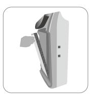
2 Place Filter 1 (Cold Catalyst and Activated Carbon. Compound Filters) back into the inner side of the product. Note: Ensure the tab side is facing you.
