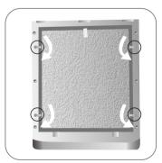
Turn the buckles to fix the filters.
