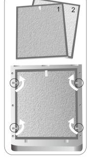
2 Turn the buckles as the Direction of the arrow, remove the filter 1 and filter 2 in turn.
